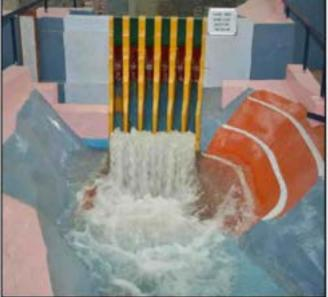
Performance of Ski-Jump Bucket for Gated Operation of Spillway for the Discharge of 3250 m<sup>3</sup>/s (25%) at FRL EI, 755 m
