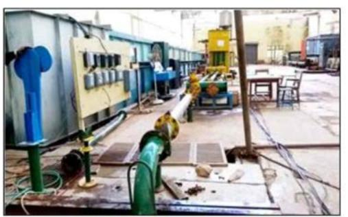
Pump Test Circuit -Piping and Volumetric Tank
