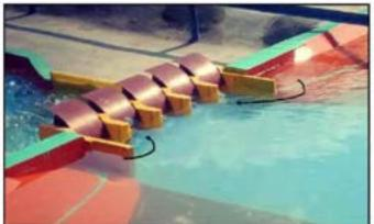
Flow Condition for Ungated Operation of Additional Spillway near the Left and Right Training Wall for the Discharge of 9122 m3/s
