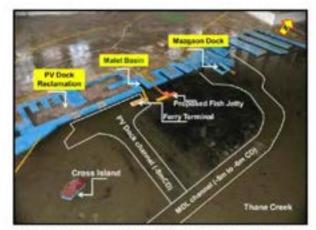
Fig. 2: Recommended Alignment of New Fish Jetty for Mumbai Port
