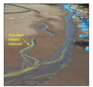
Generalized Flow Patterns near Activated Central Channel 4 Km Downstream of Kosi Barrage for Discharge of 5663 M3/s
