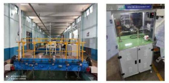
Upgradation of Current meter trolley for Calibration and performance testing of Current meter, ADCP, side looking sensor
