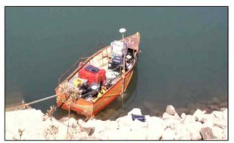
Survey Boat with Eco-Sounder, GPS with Antenna Holding by Mechanical Fixture
