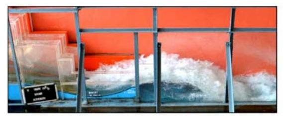
Flow conditions over the spillway and energy dissipator (Q = 8750 m3/s (100%), ungated operation of spillway)
